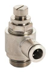
NITRA pneumatic push-to-connect fitting, elbow flow control valve, rotating, meter-out, nickel-plated brass body, nickel-plated brass threads, (1) G1/2 male BSPP to (1) 3/8in push-to-connect. Package of 2.
