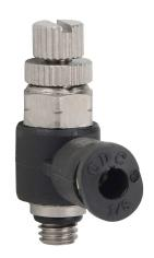
NITRA pneumatic push-to-connect fitting, elbow flow control valve, rotating, meter-out, thermoplastic (PBT) body, nickel-plated brass threads, 1/8in tube to #10-32 threaded connection(s). Package of 2.
