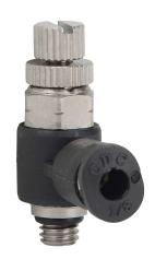
NITRA pneumatic push-to-connect fitting, elbow flow control valve, rotating, meter-out, thermoplastic (PBT) body, nickel-plated brass threads, (1) #10-32 male UNF to (1) 1/8in push-to-connect. Package of 2.
