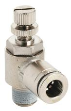
NITRA pneumatic push-to-connect fitting, elbow flow control valve, rotating, meter-out, nickel-plated brass body, nickel-plated brass threads, (1) R1/8 male BSPT to (1) 1/4in push-to-connect. Package of 2.
