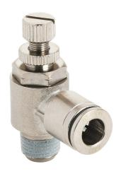
NITRA pneumatic push-to-connect fitting, elbow flow control valve, rotating, meter-out, nickel-plated brass body, nickel-plated brass threads, (1) 1/8in male NPT to (1) 1/4in push-to-connect. Package of 2.
