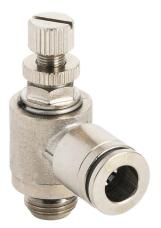
NITRA pneumatic push-to-connect fitting, elbow flow control valve, rotating, meter-out, nickel-plated brass body, nickel-plated brass threads, 1/4in push-to-connect to G1/8 BSPP. Package of 2.
