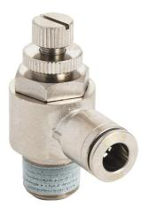
NITRA pneumatic push-to-connect fitting, elbow flow control valve, rotating, meter-out, nickel-plated brass body, nickel-plated brass threads, (1) R1/4 male BSPT to (1) 1/4in push-to-connect. Package of 2.
