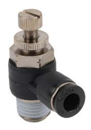
NITRA pneumatic push-to-connect fitting, elbow flow control valve, rotating, meter-out, thermoplastic (PBT) body, nickel-plated brass threads, 1/4in tube to 1/4in NPT connection(s). Package of 2.
