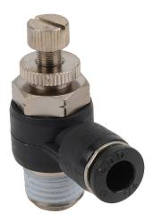
NITRA pneumatic push-to-connect fitting, elbow flow control valve, rotating, meter-out, thermoplastic (PBT) body, nickel-plated brass threads, (1) 1/4in male NPT to (1) 1/4in push-to-connect. Package of 2.
