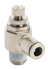
NITRA pneumatic push-to-connect fitting, elbow flow control valve, rotating, meter-out, nickel-plated brass body, nickel-plated brass threads, 1/4in push-to-connect to 1/4in NPT. Package of 2.
