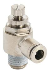
NITRA pneumatic push-to-connect fitting, elbow flow control valve, rotating, meter-out, nickel-plated brass body, nickel-plated brass threads, (1) 1/4in male NPT to (1) 1/4in push-to-connect. Package of 2.
