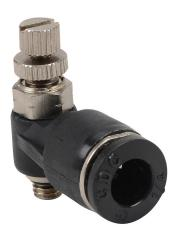
NITRA pneumatic push-to-connect fitting, elbow flow control valve, rotating, meter-out, thermoplastic (PBT) body, nickel-plated brass threads, (1) #10-32 male UNF to (1) 1/4in push-to-connect. Package of 2.
