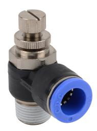
NITRA pneumatic push-to-connect fitting, elbow flow control valve, rotating, meter-out, thermoplastic (PBT) body, nickel-plated brass threads, (1) R3/8 male BSPT to (1) 12mm push-to-connect. Package of 2.
