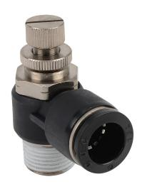
NITRA pneumatic push-to-connect fitting, elbow flow control valve, rotating, meter-out, thermoplastic (PBT) body, nickel-plated brass threads, (1) 3/8in male NPT to (1) 1/2in push-to-connect. Package of 2.
