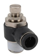
NITRA pneumatic push-to-connect fitting, elbow flow control valve, rotating, meter-out, thermoplastic (PBT) body, nickel-plated brass threads, (1) 1/2in male NPT to (1) 1/2in push-to-connect. Package of 2.
