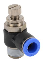
NITRA pneumatic push-to-connect fitting, elbow flow control valve, rotating, meter-out, thermoplastic (PBT) body, nickel-plated brass threads, (1) R3/8 male BSPT to (1) 10mm push-to-connect. Package of 2.
