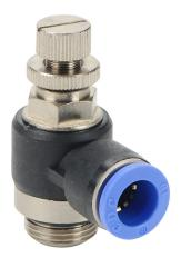
NITRA pneumatic push-to-connect fitting, elbow flow control valve, rotating, meter-out, thermoplastic (PBT) body, nickel-plated brass threads, (1) G3/8 male BSPP to (1) 10mm push-to-connect. Package of 2.
