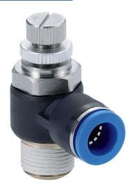
NITRA pneumatic push-to-connect fitting, elbow flow control valve, rotating, meter-out, thermoplastic (PBT) body, nickel-plated brass threads, (1) R1/4 male BSPT to (1) 10mm push-to-connect. Package of 2.
