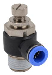
NITRA pneumatic push-to-connect fitting, elbow flow control valve, rotating, meter-out, thermoplastic (PBT) body, nickel-plated brass threads, (1) R1/2 male BSPT to (1) 10mm push-to-connect. Package of 2.
