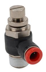
NITRA pneumatic push-to-connect fitting, elbow flow control valve, rotating, meter-in, thermoplastic (PBT) body, nickel-plated brass threads, (1) R3/8 male BSPT to (1) 5/16in (8mm) push-to-connect. Package of 2.
