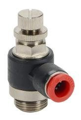
NITRA pneumatic push-to-connect fitting, elbow flow control valve, rotating, meter-in, thermoplastic (PBT) body, nickel-plated brass threads, (1) G3/8 male BSPP to (1) 5/16in (8mm) push-to-connect. Package of 2.
