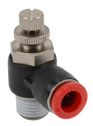
NITRA pneumatic push-to-connect fitting, elbow flow control valve, rotating, meter-in, thermoplastic (PBT) body, nickel-plated brass threads, 5/16in (8mm) tube to R1/4 BSPT connection(s). Package of 2.
