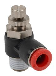
NITRA pneumatic push-to-connect fitting, elbow flow control valve, rotating, meter-in, thermoplastic (PBT) body, nickel-plated brass threads, (1) R1/4 male BSPT to (1) 5/16in (8mm) push-to-connect. Package of 2.
