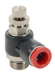
NITRA pneumatic push-to-connect fitting, elbow flow control valve, rotating, meter-in, thermoplastic (PBT) body, nickel-plated brass threads, (1) G1/4 male BSPP to (1) 5/16in (8mm) push-to-connect. Package of 2.
