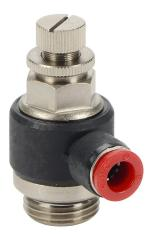
NITRA pneumatic push-to-connect fitting, elbow flow control valve, rotating, meter-in, thermoplastic (PBT) body, nickel-plated brass threads, (1) G1/2 male BSPP to (1) 5/16in (8mm) push-to-connect. Package of 2.
