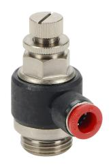
NITRA pneumatic push-to-connect fitting, elbow flow control valve, rotating, meter-in, thermoplastic (PBT) body, nickel-plated brass threads, 5/16in (8mm) tube to G1/2 BSPP connection(s). Package of 2.
