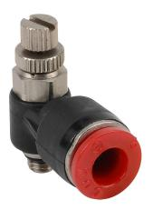
NITRA pneumatic push-to-connect fitting, elbow flow control valve, rotating, meter-in, thermoplastic (PBT) body, nickel-plated brass threads, (1) M5 x 0.8 male ISO to (1) 6mm push-to-connect. Package of 2.
