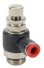
NITRA pneumatic push-to-connect fitting, elbow flow control valve, rotating, meter-in, thermoplastic (PBT) body, nickel-plated brass threads, (1) G3/8 male BSPP to (1) 6mm push-to-connect. Package of 2.
