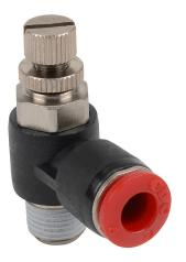
NITRA pneumatic push-to-connect fitting, elbow flow control valve, rotating, meter-in, thermoplastic (PBT) body, nickel-plated brass threads, (1) R1/8 male BSPT to (1) 6mm push-to-connect. Package of 2.
