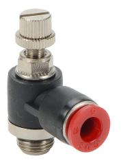
NITRA pneumatic push-to-connect fitting, elbow flow control valve, rotating, meter-in, thermoplastic (PBT) body, nickel-plated brass threads, (1) G1/8 male BSPP to (1) 6mm push-to-connect. Package of 2.
