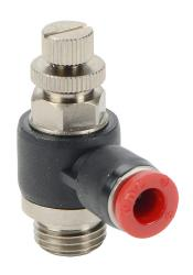
NITRA pneumatic push-to-connect fitting, elbow flow control valve, rotating, meter-in, thermoplastic (PBT) body, nickel-plated brass threads, 6mm tube to G1/4 BSPP connection(s). Package of 2.
