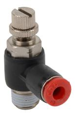
NITRA pneumatic push-to-connect fitting, elbow flow control valve, rotating, meter-in, thermoplastic (PBT) body, nickel-plated brass threads, (1) 1/8in male NPT to (1) 5/32in (4mm) push-to-connect. Package of 2.
