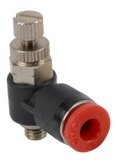
NITRA pneumatic push-to-connect fitting, elbow flow control valve, rotating, meter-in, thermoplastic (PBT) body, nickel-plated brass threads, (1) #10-32 male UNF to (1) 5/32in (4mm) push-to-connect. Package of 2.
