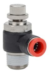
NITRA pneumatic push-to-connect fitting, elbow flow control valve, rotating, meter-in, thermoplastic (PBT) body, nickel-plated brass threads, (1) 3/8in male NPT to (1) 5/16in (8mm) push-to-connect. Package of 2.
