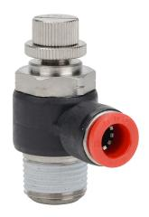
NITRA pneumatic push-to-connect fitting, elbow flow control valve, rotating, meter-in, thermoplastic (PBT) body, nickel-plated brass threads, 5/16in (8mm) tube to 3/8in NPT connection(s). Package of 2.
