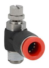
NITRA pneumatic push-to-connect fitting, elbow flow control valve, rotating, meter-in, thermoplastic (PBT) body, nickel-plated brass threads, (1) 1/8in male NPT to (1) 5/16in (8mm) push-to-connect. Package of 2.
