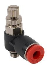
NITRA pneumatic push-to-connect fitting, elbow flow control valve, rotating, meter-in, thermoplastic (PBT) body, nickel-plated brass threads, (1) M5 x 0.8 male ISO to (1) 5/32in (4mm) push-to-connect. Package of 2.
