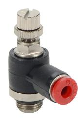
NITRA pneumatic push-to-connect fitting, elbow flow control valve, rotating, meter-in, thermoplastic (PBT) body, nickel-plated brass threads, (1) G1/8 male BSPP to (1) 5/32in (4mm) push-to-connect. Package of 2.
