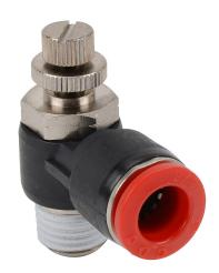
NITRA pneumatic push-to-connect fitting, elbow flow control valve, rotating, meter-in, thermoplastic (PBT) body, nickel-plated brass threads, (1) 1/4in male NPT to (1) 3/8in push-to-connect. Package of 2.
