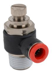
NITRA pneumatic push-to-connect fitting, elbow flow control valve, rotating, meter-in, thermoplastic (PBT) body, nickel-plated brass threads, (1) 1/2in male NPT to (1) 3/8in push-to-connect. Package of 2.
