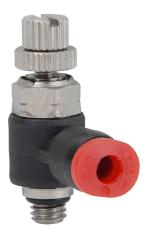
NITRA pneumatic push-to-connect fitting, elbow flow control valve, rotating, meter-in, thermoplastic (PBT) body, nickel-plated brass threads, (1) #10-32 male UNF to (1) 1/8in push-to-connect. Package of 2.
