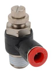
NITRA pneumatic push-to-connect fitting, elbow flow control valve, rotating, meter-in, thermoplastic (PBT) body, nickel-plated brass threads, (1) 1/4in male NPT to (1) 1/4in push-to-connect. Package of 2.
