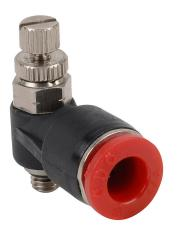
NITRA pneumatic push-to-connect fitting, elbow flow control valve, rotating, meter-in, thermoplastic (PBT) body, nickel-plated brass threads, (1) #10-32 male UNF to (1) 1/4in push-to-connect. Package of 2.
