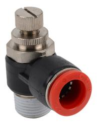
NITRA pneumatic push-to-connect fitting, elbow flow control valve, rotating, meter-in, thermoplastic (PBT) body, nickel-plated brass threads, (1) R3/8 male BSPT to (1) 12mm push-to-connect. Package of 2.
