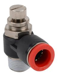
NITRA pneumatic push-to-connect fitting, elbow flow control valve, rotating, meter-in, thermoplastic (PBT) body, nickel-plated brass threads, (1) 3/8in male NPT to (1) 1/2in push-to-connect. Package of 2.
