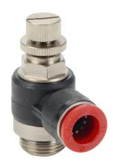
NITRA pneumatic push-to-connect fitting, elbow flow control valve, rotating, meter-in, thermoplastic (PBT) body, nickel-plated brass threads, (1) G3/8 male BSPP to (1) 10mm push-to-connect. Package of 2.
