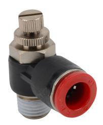
NITRA pneumatic push-to-connect fitting, elbow flow control valve, rotating, meter-in, thermoplastic (PBT) body, nickel-plated brass threads, 10mm tube to R1/4 BSPT connection(s). Package of 2.
