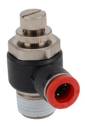
NITRA pneumatic push-to-connect fitting, elbow flow control valve, rotating, meter-in, thermoplastic (PBT) body, nickel-plated brass threads, (1) R1/2 male BSPT to (1) 10mm push-to-connect. Package of 2.
