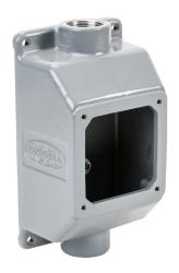
Bryant feed through back box, (2) 1in female NPT conduit entries, cast aluminum housing, gray. For use with Bryant 20A and 30A devices. Requires AP2030 adapter plate.
