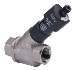
ProSense liquid flow switch, spring-supported piston, 3/4in female NPT process connection, 0.26 to 6.6 GPM, Output: switch PNP, N.O., 20.4 to 26.4 VDC operating voltage.
