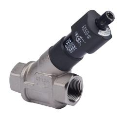
ProSense liquid flow switch, spring-supported piston, 3/4in female NPT process connection, 0.26 to 6.6 GPM, Output: switch PNP, N.O., 20.4 to 26.4 VDC operating voltage.
