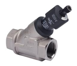
ProSense liquid flow switch, spring-supported piston, 1in female NPT process connection, 1.32 to 26.4 GPM, Output: switch PNP, N.O., 20.4 to 26.4 VDC operating voltage.
