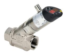
ProSense liquid digital flow sensor, spring-supported piston, 3/4in female NPT process connection, 0 to 6 GPM, 14 to 212 deg F, Output: switch or frequency, Output 2: switch or current, 18-30 VDC operating voltage.
