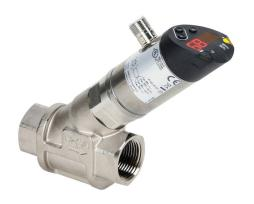
ProSense liquid digital flow sensor, spring-supported piston, 3/4in female NPT process connection, 0 to 10 GPM, 14 to 212 deg F, Output: switch or frequency, Output 2: switch or current, 18-30 VDC operating voltage.
