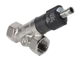
ProSense liquid flow transmitter, spring-supported piston, 3/4in female NPT process connection, 0 to 6 GPM, Output: analog, 4-20 mA, 18 to 32 VDC operating voltage.
