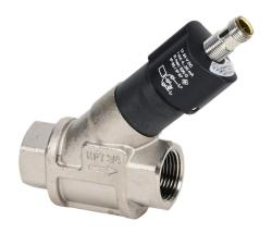
ProSense liquid flow transmitter, spring-supported piston, 3/4in female NPT process connection, 0 to 6 GPM, Output: analog, 4-20 mA, 18-32 VDC operating voltage.
