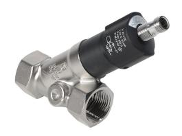
ProSense liquid flow transmitter, spring-supported piston, 3/4in female NPT process connection, 0 to 10 GPM, Output: analog, 4-20 mA, 18 to 32 VDC operating voltage.
