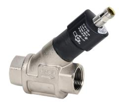
ProSense liquid flow transmitter, spring-supported piston, 3/4in female NPT process connection, 0 to 10 GPM, Output: analog, 4-20 mA, 18-32 VDC operating voltage.
