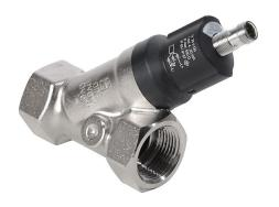
ProSense liquid flow transmitter, spring-supported piston, 1in female NPT process connection, 0 to 27 GPM, Output: analog, 4-20 mA, 18 to 32 VDC operating voltage.
